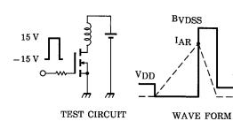
$$\begin{split} R_G &= 25~\Omega \\ V_{DD} &= 25~V,~L = 339~\mu H \end{split} \qquad EAS = 0. \end{split}$$
